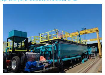
transportation of the tanks by trucks and provide mobility to relocate them to different land drilling sites.
