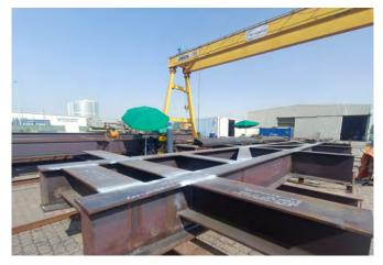
The tanks include two mixing tanks, a suction tank, a water tank, a trip tank and a separation tank. A self-elevating trailer assembly will be used in order to transport the tanks by trucks and to allow mobility to move the tanks to different land drilling wells.
