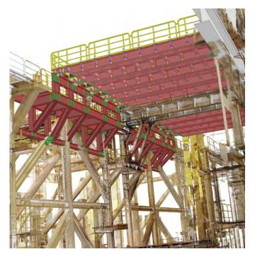
and nearly 200 square meters (2150 square feet) of deck space. The bridges are removable and stackable, allowing for storage and transport in a standard shipping container.
