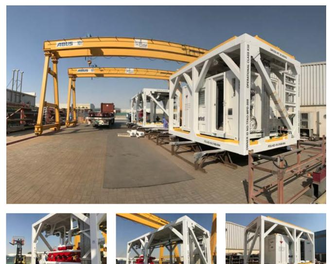
Following the experience of Fatih's MPD integration, 3C Metal implemented the same design for the Yavuz - four DNV 2.7-3 modules on the existing X-Mas tree footings, minimizing modifications required for the rig's existing structures. The team was able to do an as-built laser scan of the Fatih installation. This allowed for small touch-ups for the new installation and overall improved the efficiency for the engineering, fabrication and installation.
