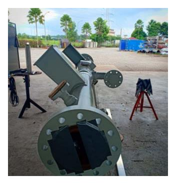
3C Metal Asia was requested to assist with the preparation of fabrication drawings as well as the supply of material (API 5L X60 grade) and fabrication of a pig receiver.
