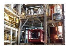
The rig's previous MPD manifolds were removed following the end of the Brazil assignment and a new set of manifolds were mobilized for the next MPD campaign in Malaysia. The rig's MPD tower was modified to accommodate the new set as well as most of the piping, which was replaced and upgraded to meet the functionalities of the new system. Additions included coriolis meters, which were fitted on all mud pumps, as well as modifications to some of the flowpath.
