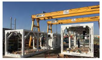
This is the fifth MPD system integration where 3C Metal has used the semi-permanent modular design for the MPD system. The versatile design involves placing four DNV 2.7-3 modules on the existing X-Mas tree footings, minimizing modifications required for the rig's existing structures. Using knowledge from previous MPD integrations and improved laser scanning technology, 3C Metal were able to gain over 150 scans of the DSMII in order to make an accurate model for the work.
