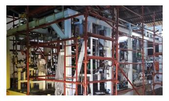
The purification unit will be used to remove non-generable salts (also called heat stable salts, or HSS) and fine particulates that accumulate in a lean absorbent fluid. The purification allows for the fluid to be recycled into the plant. The purification unit is to be commissioned as part of a new oil field operation in the Middle East.
