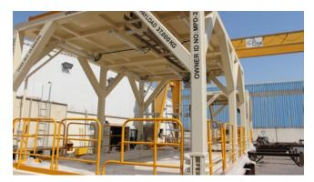
The drillship was previously equipped with a temporary Weatherford MPD system. Weatherford commissioned 3C Metal to carry out the structural and interconnecting piping components for the integration of the permanent Weatherford MPD system. The new set up will accommodate the IWOCS and the Weatherford MPD system onboard.
