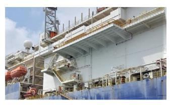
3C Metal was also involved in other upgrades during the voyage. A rope access team worked on adding more than 50 new latches to the belly board. Some light platforms were also installed on the side of the helideck to accommodate two helicopter approach path indicators (HAPIs).
